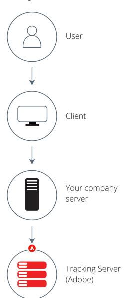
Sending the data from your own server has the advantage of gaining full control over the data sent to Adobe. You can add or remove data from the analytics payload.
